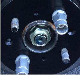
3. Install hubs onto the spindles using the previously removed load washers and nuts. Tighten the nuts to 139 LB-FT and then stake them into the notches in the spindles as shown in the above-right image.
